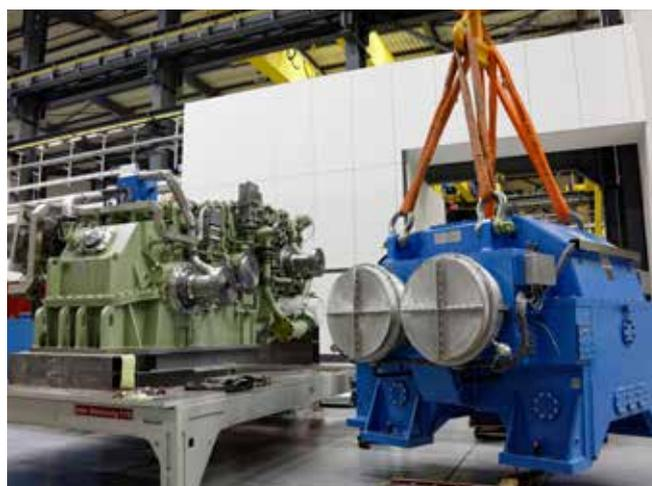
Intermediate gear; ratio = 4.037/6.776; 12 MW; 500,000 Nm
