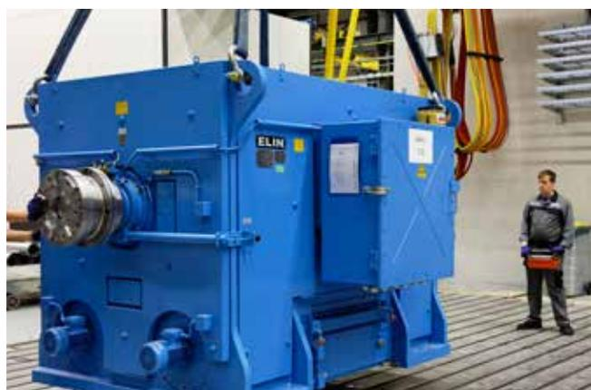
AC-Motor; 6 MW; 2,400 rpm; 38,000 Nm
