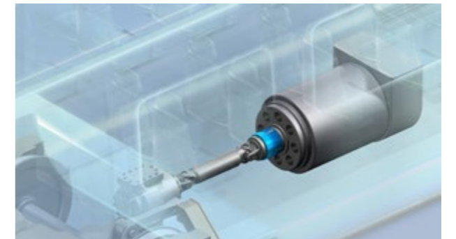
Drive unit of a high-speed train
