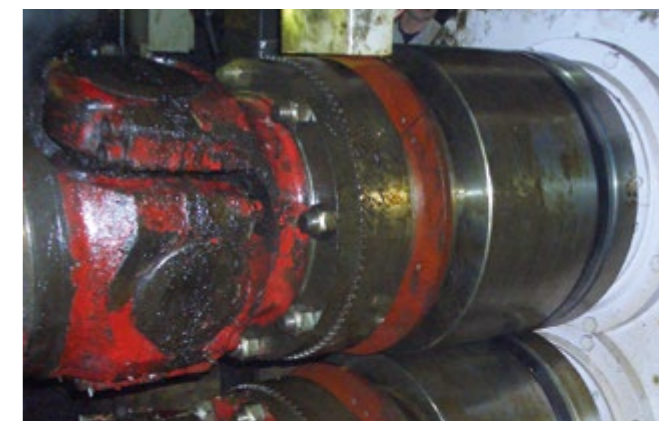
HYGUARD® safety coupling type HDW 300 with torque measurement system in a cold rolling mill after years of service
