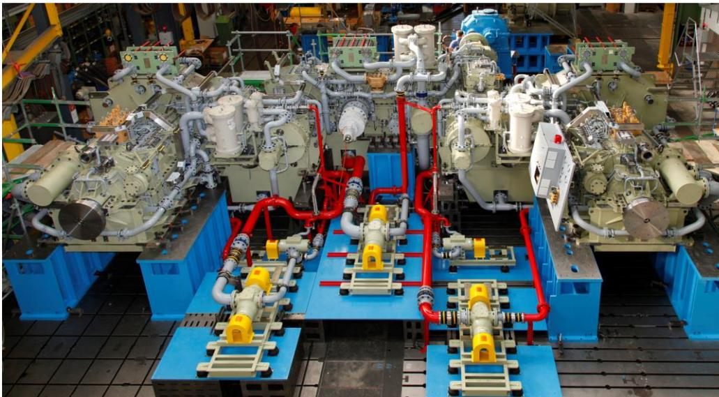
**Fig. 3:** The F125 RENK CODELAG gear system with cross connect gear (center) and port and starboard main gears, view from forward. Clutch arrangements in front of main gears.
